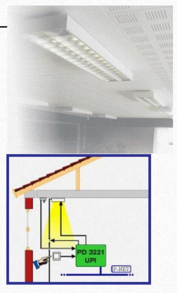
All inputs and outputs are connected to a UPI module having a combined calculator and pulse-processor program installed, which internally carries out the required regulation. Setpoints are uploaded from elsewhere, via P-NET.
