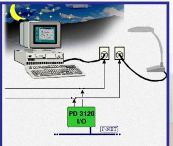
**P-NET controlled power outlets** Power turned off when enabling alarm **Backup by night**
